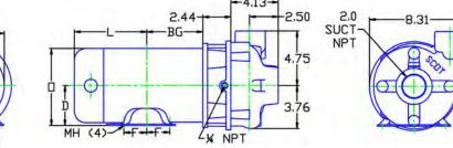
ALL DIMENSIONS IN INCHES. DRAWING REPRESENTS APPROXIMATE PUMP DIMENSIONS. AUTOCAD DRAWING TO SCALE ABAILABLE FROM FACTORY.
