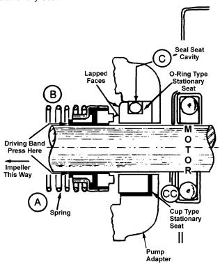
**CAUTION:** Never operate the lapped running faces dry. The liquid being handled ensures proper lubrication.
