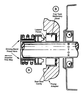
**CAUTION:** Never operate the lapped running faces dry. The liquid being handled ensures proper lubrication.
